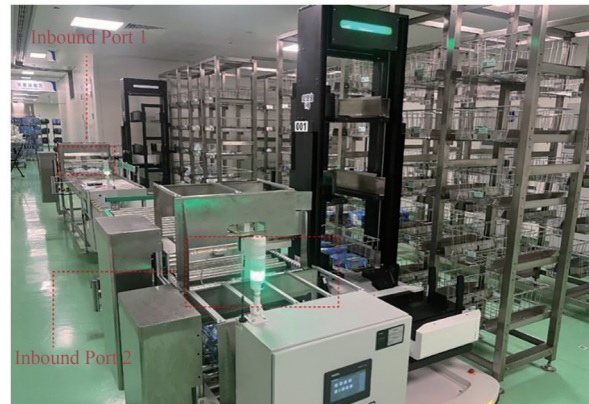
Figure 4 Schematic diagram of dual-robot operation during inbound tasks under a dual inbound port configuration
